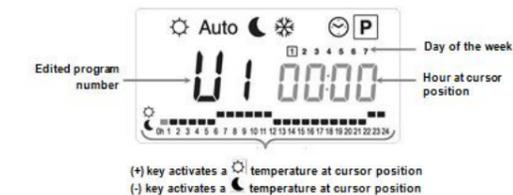
With navigation keys (◀) and (▶), move the blinking cursor on the hour of the day that you want to modify. When the day seems to be correctly edited, press (OK) key.
