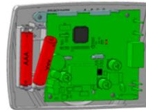
> Close the thermostat by placing the front face in front of the rear face and push on it to lock:
